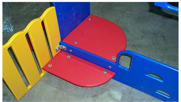
9. Now install the flower pot (N) and the flower (O) to the front entry panel using 5/16" x 1 ½" button head bolts, 5/16" x 1" button head nuts, 5/16" flat washers, and 3/8" flat washers.
