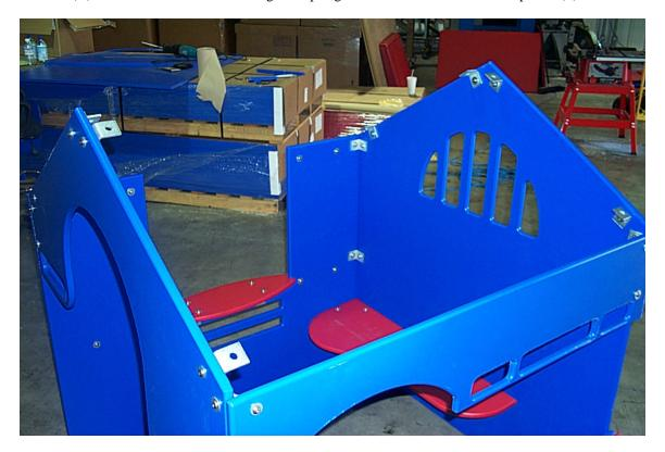
16. Now install 1 of the 2 roof panels with 5/16" x ¾" button head bolts, 5/16" x 1" button head nuts, 5/16" flat washers, and 3/8" flat washers. Be sure that the beveled edge is toward the peak of the roof. Do not tighten at this time. Repeat for the second roof panel. Once both panels are in place align both roof panels together, flush at the top and tighten all hardware. This can be difficult and may take a couple of adjustments to make them meet tightly together.
