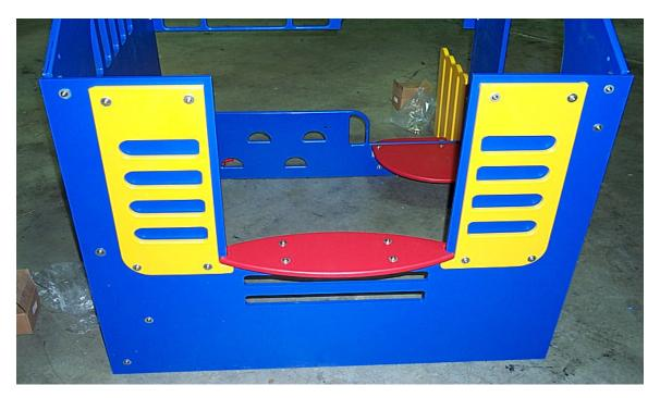
12. Now remove the 2 bolts holding the lower side panel to the back panel (A) and install 2 corner brackets in the same place with the corner turning toward the front of the structure. Now install 2 more corner brackets to the remaining 2 holes in the lower side panel with the corner turning towards the back of the structure. See picture below. These brackets are for the ladder support triangles (L).
