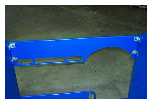
6. Install 3 corner brackets in the lower 3 holes of the back panel (A) and 1 bracket on the side counter panel (B) near the back towards the back panel (A). Now attach the large seat (F) on these 4 brackets with 5/16" x 3/4" bolt, 5/16" x 1" nut, 5/16" washer, and 3/8" washer and tighten all hardware along this side, making sure the corners are flush with one another.
