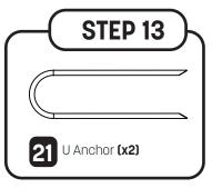
Now place one side of the included U anchors (21) into the holes in the feet of the Jungle Line. Place the anchors so the angle away from the jungle line as shown. Use a hammer or rubber mallet to push the anchors (21) firmly into the ground.
