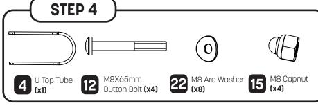
Now place the U top tube **(4)** onto the uprights **(1)** and secure together with four M8X35mm button bolts **(12)**, eight M8 arc washers **(22)** and four M8 capnuts **(15)**.
