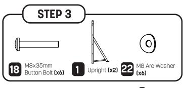
Place the two uprights (1) on the ground as shown. Then line up the three cross bars (4) from step two with the holes in the uprights (1) and place them between them. Secure in place with six M8X35mm button bolts (18) and six M8 are washers (22). **Do not tighten the locknuts.**
