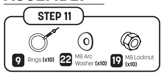
Attach the ten rings (9) through the holes in the now assembled tube section. Secure them in place with ten M8 arc washers (22) and ten M8 locknuts (19) as shown.
