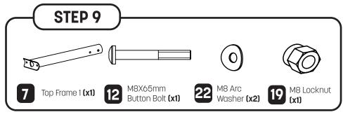
Attach the top Frame 1 (7) to the connection tube (10) on the left. Secure in place with one M8X65mm button bolt (12), two M8 arc washers (22) and one M8 locknut (19).
