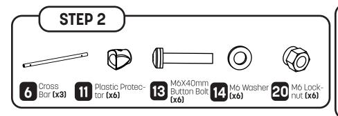
Attach two plastic protectors (11) to either side of a cross bar (6) with two M6X40mm button bolts (13), two M6 washers (14) and two M6 locknuts (20). Repeat this step until the remaining two cross bars are assembled.
