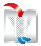
The fine filter system GENIUS-X<sup>2</sup>, with integrated pre-washing process, filters the wash water continuously and then pumps out the soil particles.
