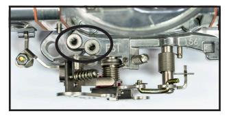
**STEP TWO**Install spring perch on to throttle body, using the two mounting holes.
