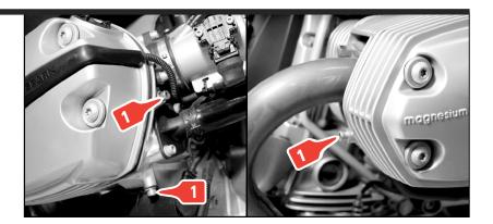
2. Position an X-Head over the cylinder head, aligning the mounting holes with the bosses on the engine.
