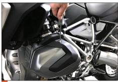
1 Remove one T25 Torx screw retaining the spark plug cover. Remove cover.
