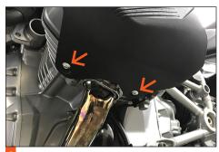
Fasten the X-Head with the supplied T25 Torx screws, starting at the bottom. *Do not tighten!*Be careful not to cross-thread the screws.
