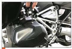
Align the upper mounting hole with the mount on the engine, and fasten with one T25 Torx screw.
