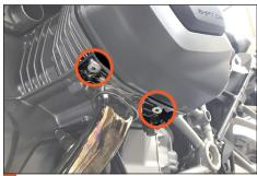
**2** Before installation, identify the two lower mounting points.
