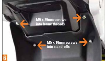
**Add a washer to each M5 Torx head screw.** Insert an M5 x10 screw through the MudSling and into each stand-off, and an M5 x 25 screw through the rear holes of the MudSling into the frame threads. Tighten all screws with a T25 Torx driver.
