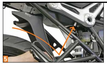
**Position the MudSling forward and low**, then lift to align its mounting holes with the Stand-offs and rear mounting holes.
