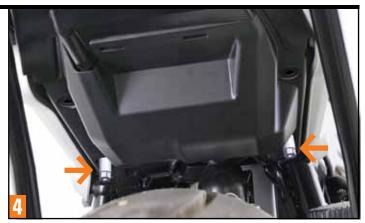
**Install the supplied stand offs** into the two forward most mounting locations. Tighten using a 10mm wrench.
