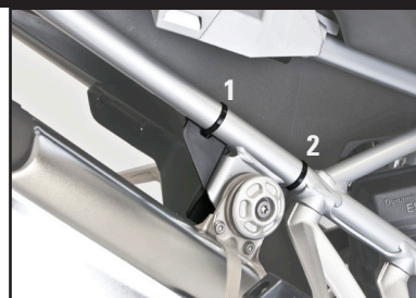
7 Position the right side wing against the exhaust mount. Install zip ties up from the bottom through the slots, around the frame and in through the outside slots.
