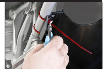
9 Cut off excess zip tie length with a wire cutter for best appearance.
