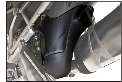
3 Position the MudSling "shoe" below the existing fender & pull up to engage it. Shown here with wheel removed.
