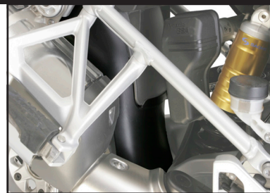
4 View from right side of bike: MudSling is shown properly engaged with the end of the fender.
