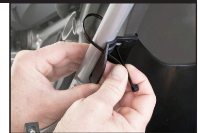
6 Loop the zip tie around the frame and back in through the slot on the outside. Pull zip tie tight. Install second zip tie.
