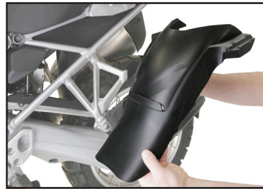
1 Hold the MudSling next to the bike in the direction of installation.
