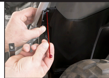
5 Hold the left side wing of the MudSling against the frame. Insert first zip tie up from the bottom through a slot. Zip tie head faces the tire.
