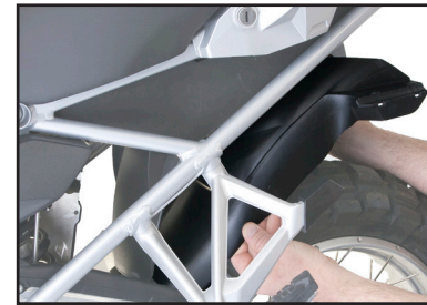
2 Place MudSling above rear tire and under the existing fender.
