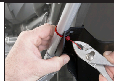
8 After pulling the zip ties as tightly as possible by hand, use pliers to tighten all zip ties fully.
