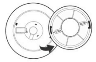
Remove cap to expose screw base.
