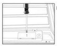
Remove the wire connection cover on the foture, by using a phillip screwdriver.
