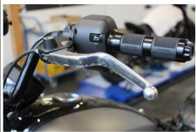
Completely remove the original lever.
