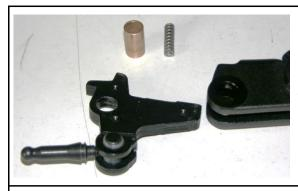
Carefully disassemble the original lever.
