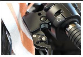
Mount the lever to the housing using the original the bolt (on the clutch lever mount the cable first).
