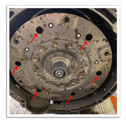
The weld-inserts are mounted in the six holes marked with the red arrow.
