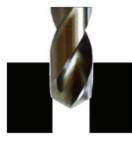
If necessary countersink the borehole.
