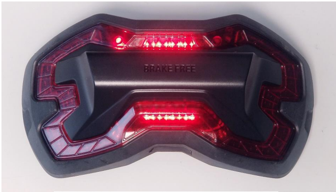
Brake Free in Low Battery Mode
