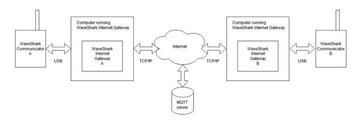
The WaveShark Internet Gateway software running on a computer connected to the Internet and connected to a WaveShark Communicator via USB will be condensed into the following icon in all subsequent diagrams in order to condense the size of said diagrams and to allow us to explore bigger ideas:
