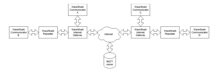
A WaveShark Internet Gateway in range of a number of WaveShark Communicator and WaveShark Repeater devices (a local WaveShark network with an Internet Gateway) will be condensed into the following icon in all subsequent diagrams in order to condense the size of said diagrams and to allow us to explore bigger ideas:
