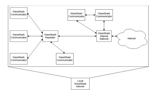
The diagram below shows a handful of local WaveShark networks interconnected via WaveShark Internet Gateways:
