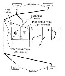
Yamaha Basic 36-Volt Wiring Diagram
