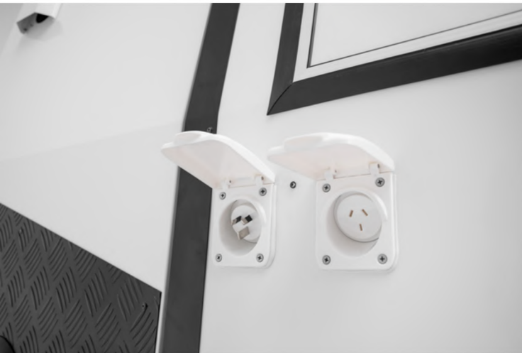
IP44 MAINS POWER INLET & INVERTER OUTLET
