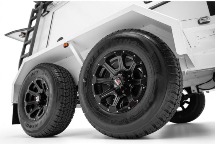
16" ALLOYS - LT 265/75R 16 TYRES FITTED TO LANDCRUISER 6-STUD HUBS
