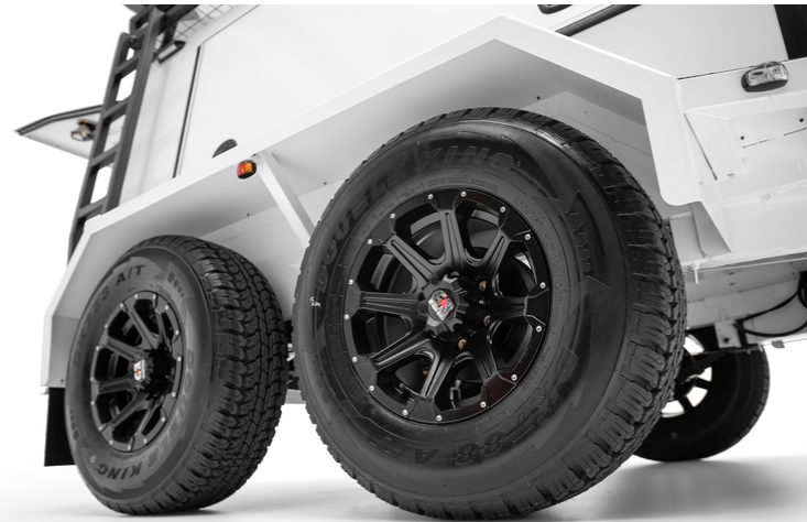
16" ALLOYS 265/75R 16 LT FITTED TO LANDCRUISER 6 BOLT HUBS
