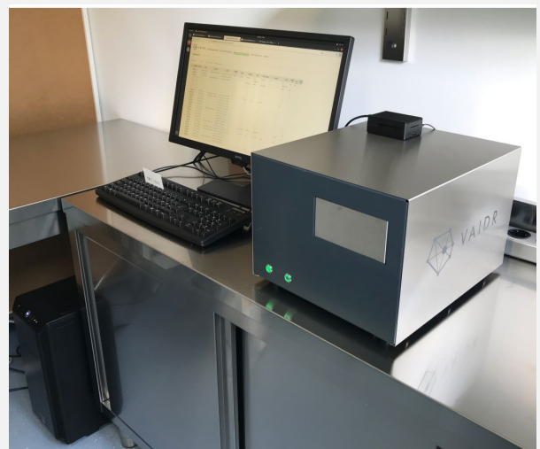
Fig. 2: VAIDR System composed of plate reader microscope and image analysis station.
