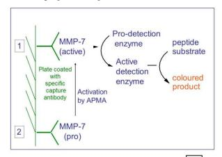
Active MMP-7: direct measurement 1 Pro-MMP-7: measurement after activation with APMA 2
