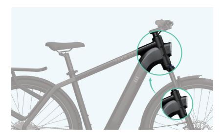
Take out the front carrier and accessory kit, use the No.4 Hex Key to tighten the screw, and install the flat washer, front carrier, and head tube in sequence. (Torque: 4–5 Nm) Pay attention to the location of the front brake hose.
