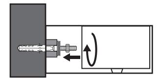
**Step 5.** Screw a metal nut onto each fixing bolt to secure the basin.
