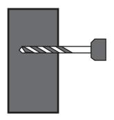
**Step 1.** Drill two holes in the required position on the wall using a  $\phi 0.55''$  masonry drill bit. The hole depth is 2.95".
