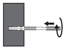
**Step 3.** Screw a fixing bolt into each fixing plug using a 0.31" spanner until the spanner contacts the wall.
