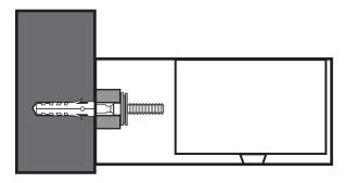
**Step 4.** Place the basin in position against the wall. Put the fixing bolts through the rear holes of the basin. Place a plastic washer, then a metal washer, onto each fixing bolt.
