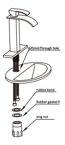
2. Make sure the basin has a  $\phi$ 35mm through hole, pass the hose through thehole, pass the rubber ring, rubber washer, and fixing nut into the hose in theorder of the drawing, and tighten the fixing nut and the fixing screw to fix the faucet on the basin
