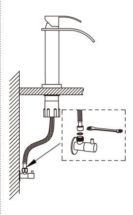
3. Connect the two inlet pipes on the main body of the faucet to the angle valve.Follow the "red" and "blue" points on the handle of the faucet, the left is red and the right is blue, respectively connecting the "hot"/"cold" water.
