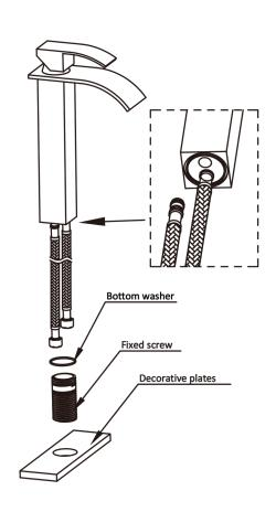
1. Connect the water inlet pipe to the faucet, then put the bottom gasket into the bottom of the faucet, then tighten the faucet with a fixing screw, and then put on the decorative panel.
