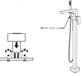
9. Once installation is complete, turn on the main water supply. Turn the faucet on and allow the water to flow for 60 seconds. Check for any leaks, and that hot and cold water are running appropriately. Divert the water to the hand shower and allow the water to flow through the hose for approximately 60 seconds
