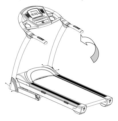
**Step 4**: Follow the arrowhead to put the plastic cover on the bottom frame, Fix the bottom cover with two bolts (ST4\*20) on either side,,then put the casket on the console.
