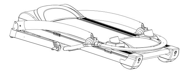
**Step 2:** Follow the arrowheads to attach the stand post(please ensure you don't put your hand on the connections), fix the stand post to the bottom frame with the 2pcs bolts M8\*50 each side. Please do not tighten all the bolts at this stage.
