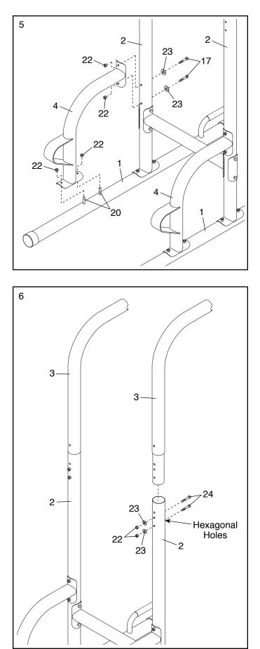
6. Orient one of the Pull-up Frames (3) as shown, and insert it into one of the Uprights (2). Attach the Pull-up Frame with two M8 x 68mm Bolts (24), two M8 Curved Washers (23), and two M8 Locknuts (22). Note: The Bolts must be inserted into the lowest set of holes in the Pull-up Frame and the Upright. Make sure that the bolt heads are in the hexagonal holes in the Upright. Do not tighten the Locknuts yet.
