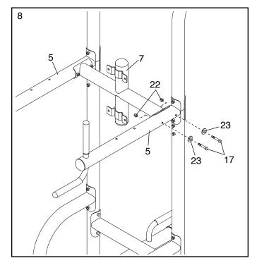
Attach the Pull-up Bar (9) to the Pull-up Frames
