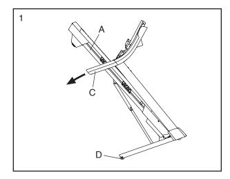
Pull back on the handrail until the treadmill will roll on the wheels, and carefully move it to the desired location. CAUTION: Do not move the treadmill without tipping it back, do not pull on the frame, and do not move the treadmill over an uneven surface.
