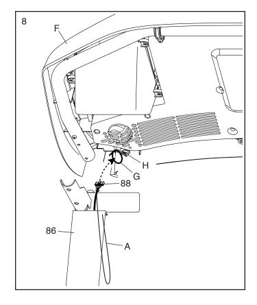
9. Set the console assembly (F) on the Right and Left Handrails (81, 80); do not pinch any wires.
