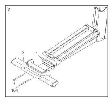
With the help of a second person, place some of the packing materials (not shown) under the front of the Frame (1). Have the second person hold the Frame to prevent it from tipping while you complete this step.
