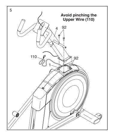
Locate the wire tie (A) in the lower end of the Upright (4). Tie the wire tie to the Upper Wire (110) as shown. Then, pull the upper end of the wire tie until the Upper Wire is routed through the Upright.
