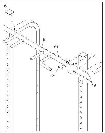
7. See steps 2–6. Tighten the M10 Locknuts (21) and the M10 x 95mm Bolts (19).
