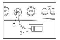
a moment, the display will light. **IMPORTANT: In an** emergency, the key can be pulled from the console, causing the walking belt to slow to a stop. Test the clip by carefully taking a few steps backward; if the key is not pulled from the console, adjust the position of the clip.
