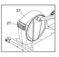
shown) from the Top Shield (37), and then use a standard screwdriver to pry the Top Shield upward off the elliptical.
