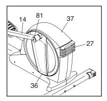
**See the lower drawing at the left.** Remove the four M4 x 16mm Screws (not shown) from the Large Storage Foot (27), and remove the Large Storage Foot. Next, remove the two M4 x 16mm Screws (not shown) from the Top Shield (37), and then use a standard screwdriver to pry the Top Shield upward off the elliptical. Then, pry the left Pedal Disc (36) off the elliptical.
