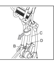
Next, push the upright (C) in the opposite direction slightly, lift the latch (D), and then lower the upright to the folded position. Hold the upright in one of the indicated locations (E) while you lower the upright; do not hold the upper body arms.
