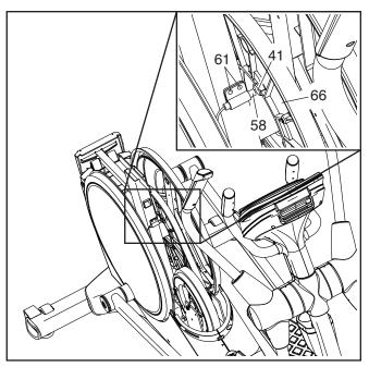
Next, slightly loosen the two indicated M4 x 16mm Screws (61). Then, slide the Reed Switch (58) slightly toward or away from the Magnet (41), and retighten the Screws.
