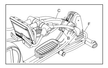
When you are finished moving the elliptical, lift the upright (C) to the vertical position and tighten the upright knob (B).
