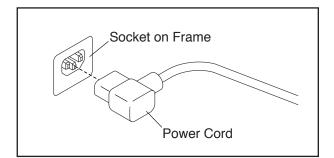
2. Plug the power cord into an appropriate outlet that is properly installed and earthed in accordance with all local codes and ordinances.
