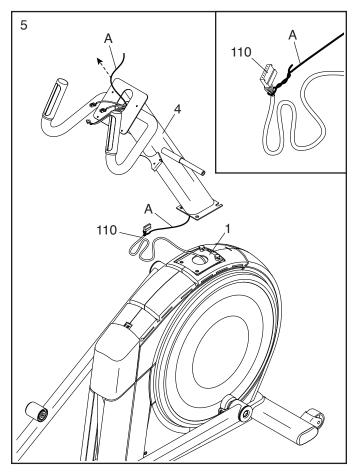
6. **Tip: Avoid pinching the Main Wire (110).** Have a second person hold the Upright (4) on the Frame (1).
