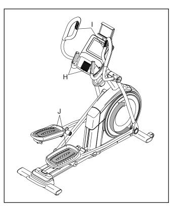
To dismount the elliptical, wait until the pedals (J) come to a complete stop. **Note: The elliptical does not have a free wheel; the pedals will continue to move until the flywheel stops.** When the pedals are stationary, step off the higher pedal first. Then, step off the lower pedal.
