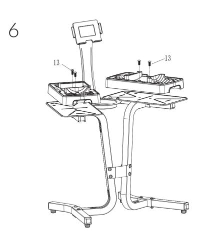
Attach the dumbbell cradles to the Dumbbell Brackets (No.9), securing with Allen Bolts (No.13).
