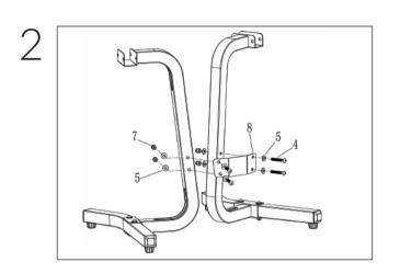
Attach the Stand Tube Connecting Plate (No.8) to the Stand Tubing (No.3), securing with 4 Allen Bolts (No.4), 8 Flat Washers (No.5) and 4 Acorn Nuts. (No.7)
