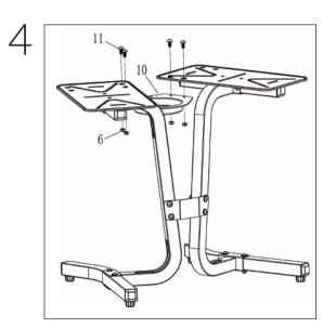
Attach the Storage Tray (No.10) to the Dumbbell Brackets (No.9) securing with 4 Allen Bolts (No.1) and 4 Lock Nuts (No.6)
