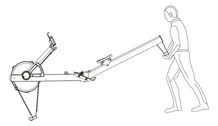
4. The Main Frame (175) and the Rail Frame (176) can be separated to minimize the unit size for storage. Remove the Pull Pin (98) from the Main Frame (175). Lift up the Main Frame (175) and pull out the Rail Frame (176) to separate. Insert the Pull Pin (98) back to the hole in the Main Frame (175) for storage.
