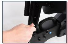
9. Tighten screws with hex key.
