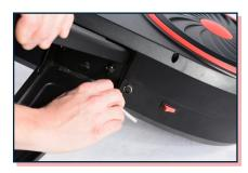
2. Tighten the screws with hex key.
