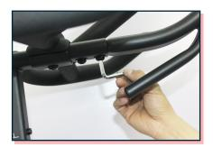
Place flat washers to table mount bolts, place table mount bolts with washers, finger tighten, then secure bolts with washers with hex key.
