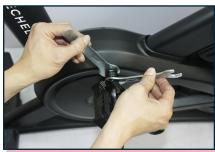
Hold pedal with double-sided wrench and use single-sided wrench to tighten nut clockwise.
