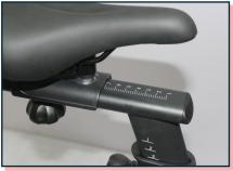
Turn the seat slide adjustment knob clockwise to secure and tighten in place.
