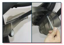
Slide water bottle holder onto post, secure both sides with screws and hex key.
