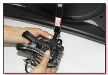
Ensure pedal and crank arm are both marked with the L Label.Screw left pedal onto left crank arm clockwise. Finger tighten nut counterclockwise back onto pedal bolt.
