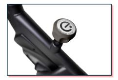
To adjust the resistance while using the Echelon® GT, turn the resistance adjustment knob to the left or right. To stop the bike press down on the resistance adjustment knob.
