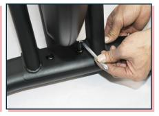
Insert foot bolts into front foot and tighten down with hex key.
