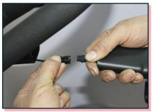
Connect the wire from the handlebar post to the wire at the bottom of the tablet mount.
