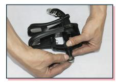
Remove nut from the right pedal by turning counterclockwise.
