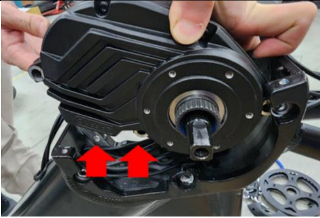
4/5) Lift up the motor to reach plugged cables.
