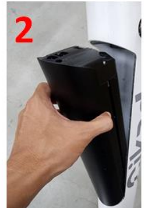
1/3) Turn the battery locking key and take off the battery from frame.
