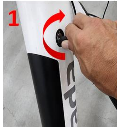
1/3) Turn the battery locking key and take off the battery from frame.
