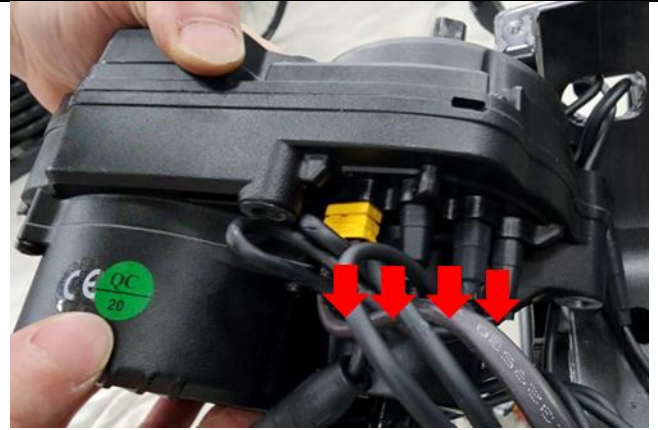
5/5) Unplug cables to take off motor.
