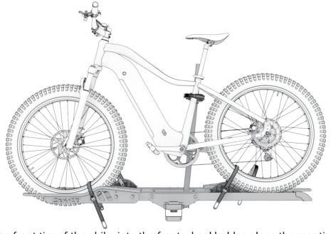
Snap the front tire of the ebike into the front wheel holder, place the rear tire in the beam, and then use the ratchet wheel straps to fix the front wheel, rear wheel, and seat/middle tube of the bike as shown in the figure below.
