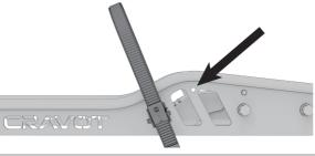
If you want to load a narrow-tire bicycle, first use an H4 hex wrench to reposition the ratchet wheel strap to the upper hole.
