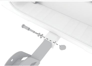
Align the holes of the folding tube with the holes on the vehicle's 2" hitch receiver. Place an **Pin Lock (16)**, through the Spring Washer and Flat Washer and the aligned holes. Insert the lock head and ensure it is securely fastened.
