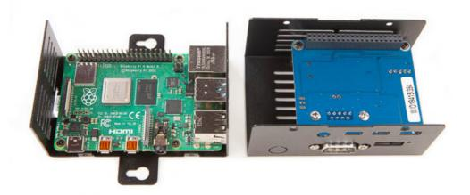
Slide the top half to the lower half. Make sure it is aligned with not gaps.
