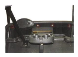
Step 12 Feed threaded end of switch though the dash where the hole was drilled. Attach the nut to secure the harness.
