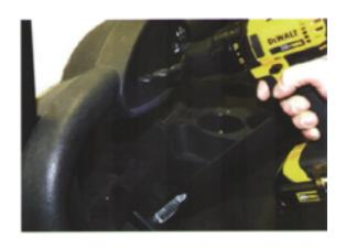
**Step 11**Unscrew the torx head screws and remove dashboard. \*\* Do not remove completely.\*\*
