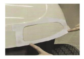
**Step 6**Drill a pilot hole and cut out shape of the headlight.
