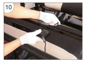
13. Match the holds on the reinforcement iron plate.
