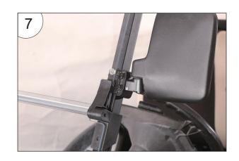
5. Install the nut on the backside of the hinged jaw slide.
