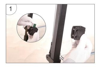
2. Install the hinged jaw slide at the proper height of the strut.
