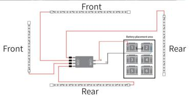
Wiring Diagram of Golf Cart Ribbon Light Bar.
