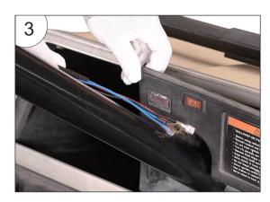
4. Let the wires and connector go through the front of the cart.
