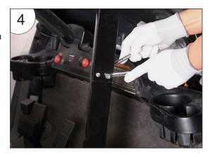
7. Choose the right position, pay attention to the hole position to avoid the chassis line and car bearing girder overlap.
