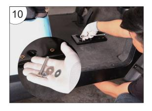
13. Remove the small screw from the cover plate by hand.
