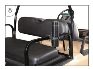
6. Tighten the 10.6mm screw of the plastic main bracket with the2.8mm diameter hex wrench.
