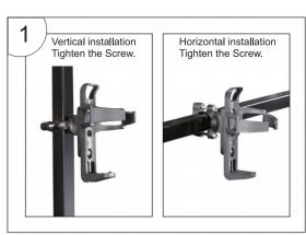
2. Adjust the bracket position that connecting the cup.
