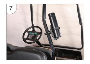
5. Tighten the 24.3mm screw of the aluminum alloy connector with the 3.7mm diameter hex wrench.
