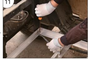
14. Secure the connection between the M8 x 30mm countersunk head screws and the front aluminum alloy plate with a cross screwdriver and a 14mm wrench.
