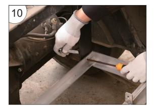
13. Secure the connection between the M8 x 30mm outer hexagon screw and the cart's crossbeam with a 14mm wrench.
