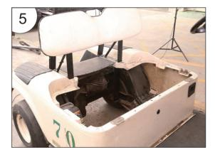
8. Grab the new battery tray and angle it into the battery hold area.
