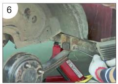
9. Install new urethane bushing and steel bushing.
