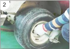
5. Raise the frame of the rear suspension with the jack to hang the rear tire in the air.
