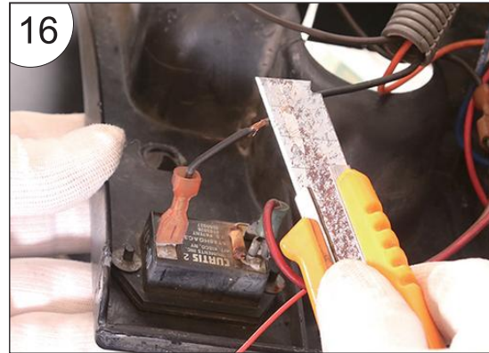
16. Strip the Original Wires of the Voltmeter (Do Not Cut).
