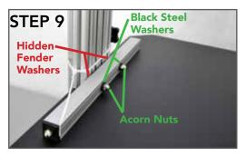
**Step 9:** Put (1) Black Washer{G} and (1) Acorn Nut{E} on the end of each of the Hex Head Bolts. Using the 7/16 wrench{H} tighten the Acorn Nuts securely. After you have the work surface secure, you can cut the zip tie holding the assembly together.
