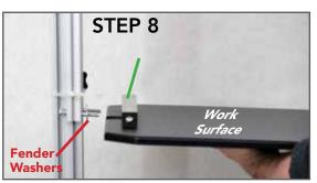
**Step 8:** Lift the Work Surface up and align the holes in the Horizontal Rail with the (2) 1/4-20 x 2.50 Hex Head Bolts{B}. Push the Work Surface onto the Hex Head Bolts until the threads of the bolts come through the Horizontal Rail.
