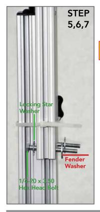
Step 5: Put (1) Locking Star Washer{I} on each of the 1/4 –20 x 2.50 Hex Head Bolts{B}.
